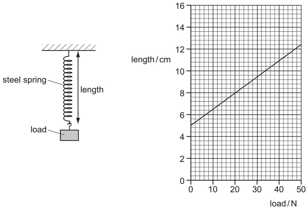
What is the extension of the spring when a load of 20 N is applied to it?
